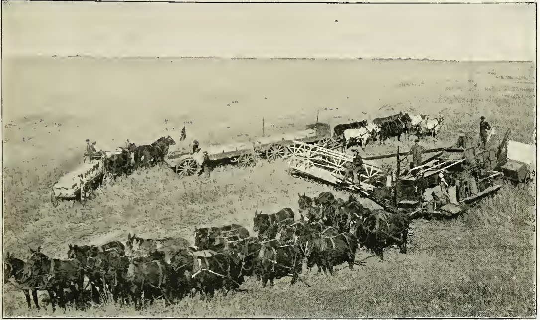
FIG. 183. — Cutting wheat in the fertile wheat region of eastern Washington. By this large machine, drawn by thirty-two mules and horses, the wheat is cut, threshed, and put into sacks ready for shipment.
